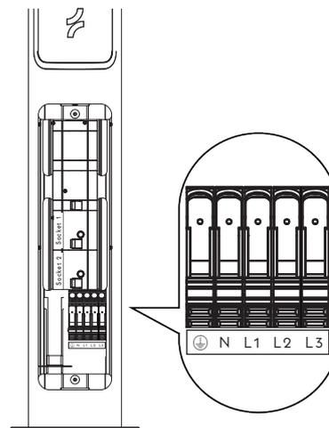
7. Close the door and secure using the H5 Pin Hex Allen Key. Ensure Earth cable is connected, remains intact and is not trapped when the door is repositioned and closed.
